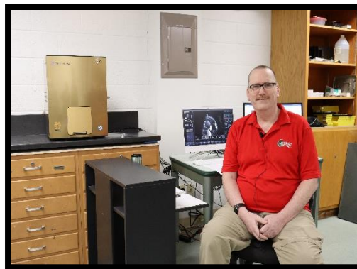
Figure II-14. Dr. Webster (MiSU) was able to purchase a Cube II SEM with EDAX Element EDS and computer systems. Click on the thumbnail to view the associated equipment video.
