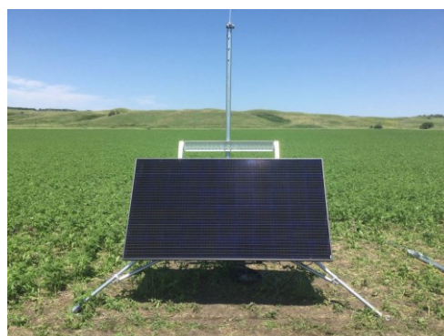
Figure II-10. Power assembly tripod component to carbon flux instrument at Tribal Demonstration Farm, Dunseith, ND.
